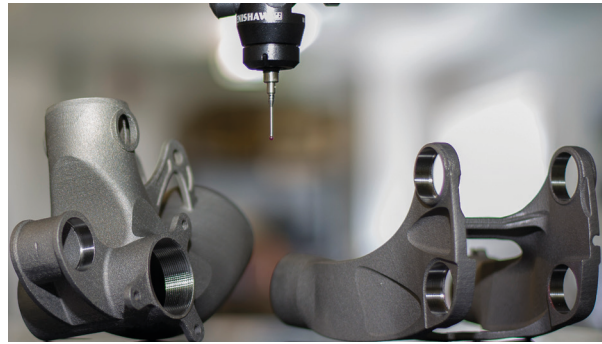
The final stage in the production of the titanium parts is inspection using Renishaw probes.
