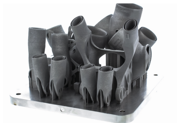
The complete set of titanium joints are produced on a single build plate on Renishaw's additive manufacturing system.
