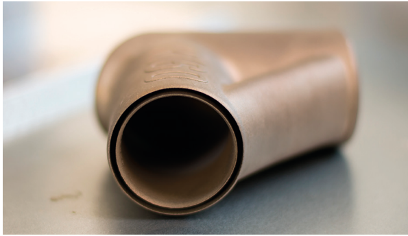
Producing the titanium parts with additive manufacturing allows double-lap shear joints to be used to join the metal lugs to the composite tubing.
